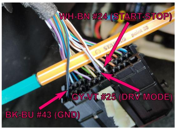
Connections can be done by soldering or special "on wire" clamps:
