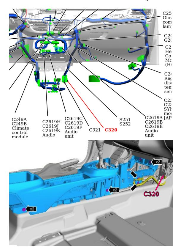
Connections to button lines and GND:
