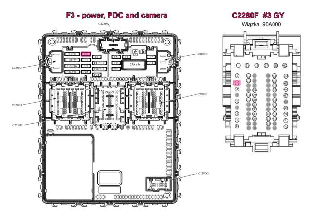
Connection to F3 fuse can be done using a fuse splitter:
