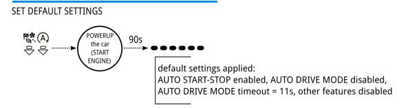
or before mounting in a car, tie to GND both the signal lines, power up with 12V and wait 90 seconds:
